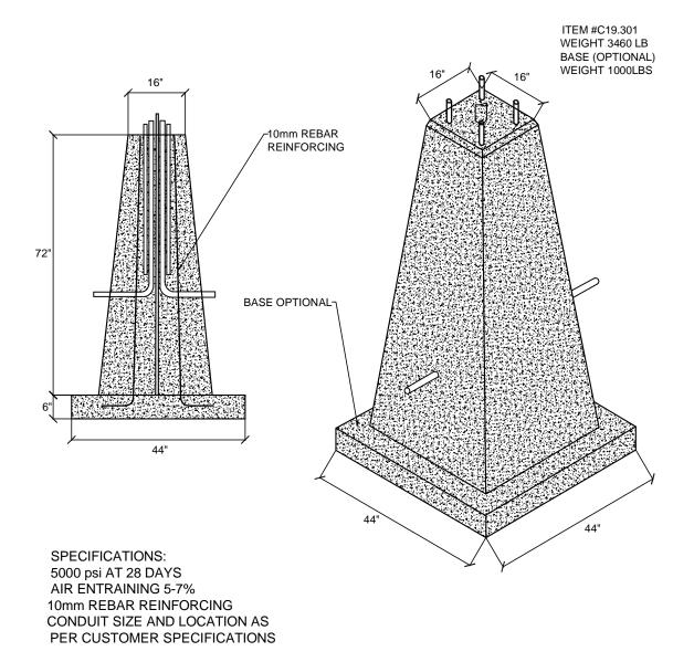
NOTES: QUICK INSTALLATION RESULTS IN MINIMAL DISRUPTION OF TRAFFIC DEPTH OF CONCRETE FOOTINGS BELOW GRADE MINIMIZES FROST MOVEMENT CAN BE PRODUCED WITH GALVANIZED CORNER PROTECTOR
